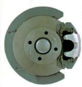
Maximum safety is assured by the front-wheel disc brakes that are paired with self-centering drums on the rear wheels.
